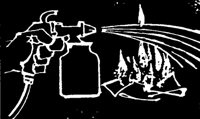
LOW-PRESSURE SPRAY TEST (AMS-3150B) —Fluid sprayed at low pressure over an ignited oil-soaked rag.
