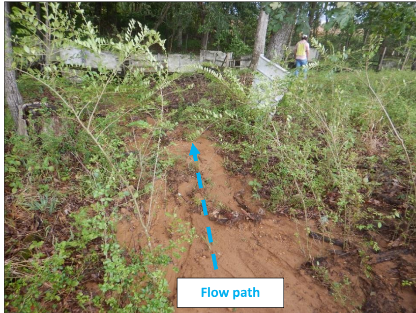
Photograph 43. View of sediment that had discharged offsite in the center of the Site. Note that the area in this picture is entirely offsite.
