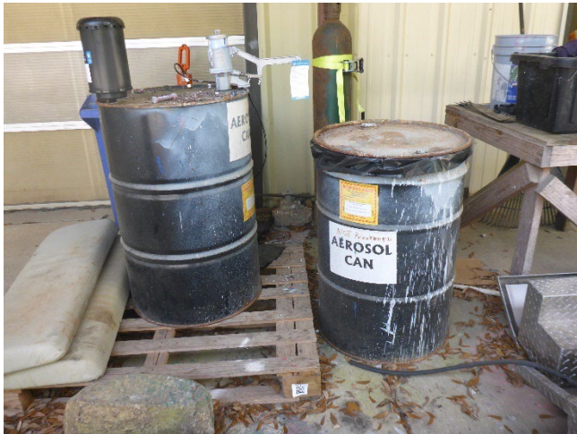
Photo 5: One 55-gallon drum of hazardous waste paint related material from puncturing aerosol cans and one 55-gallon drum of hazardous waste aerosol cans in SAAs at the Landscaping/Grounds Maintenance Area.
