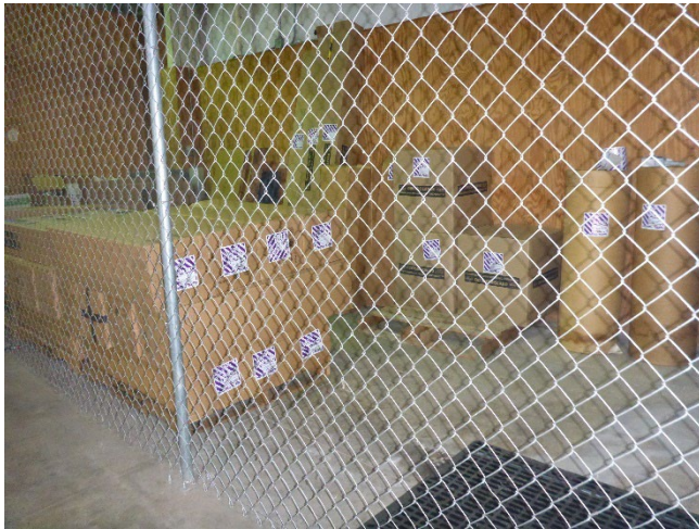
Photo 7: Two 4-foot cylinders; three 2-foot square boxes; three 4-foot boxes; three 8-foot boxes, and three pallets, each containing approximately eighteen 4-foot boxes observed in the Maintenance Division. Each box was labeled universal waste lamps and marked with an accumulation start date. Facility personnel stated that the USA ships universal waste off-site three or four times each year, and the oldest date observed on any container was April 22, 2022.
