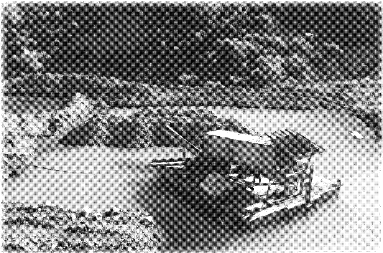
Photo 11. Small, floating “New Zealand-style” washplant from placer operation in south-central Alaska. Washplant functions similarly to the old-style bucket-line dredges, except these are usually fed via an excavator instead of a bucket line. This style of operation can reduce the amount of equipment involved to only a dozer, excavator, and the washplant; however, a good sized pond system and fairly wide valley are needed to lay out the system. PHOTO PROVIDED BY DNR, DIVISION OF MINING, LAND & WATER.
