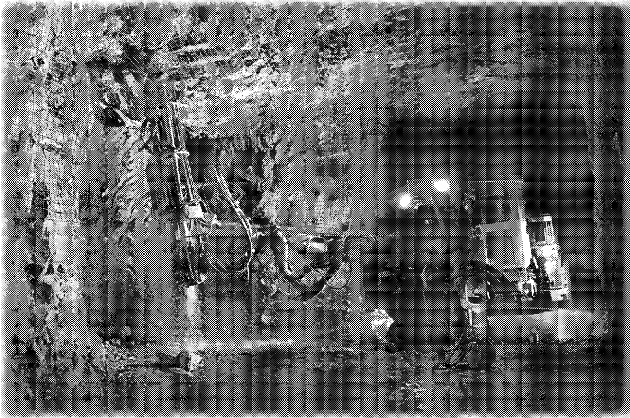
Photo 15. A roof bolter used underground at Kensington Mine to secure the roof. PHOTO PROVIDED BY COEUR ALASKA INC.
