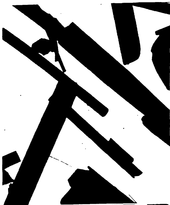
FIG. 8.—Electron micrograph of glass fibre ( \times 1875 ). 10 \mu m
