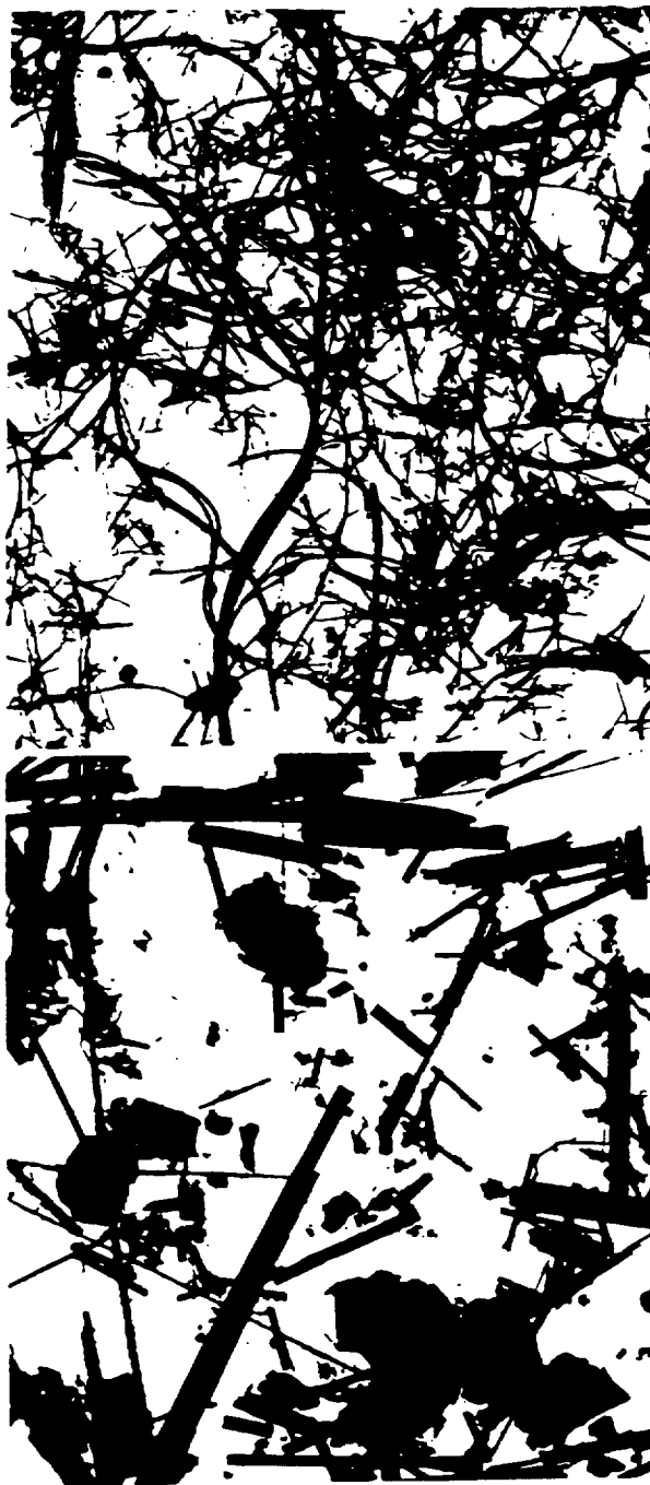
FIG. 6. Electronmicrograph of UIC + Canadian chrysotile ( \times 1875 ).
