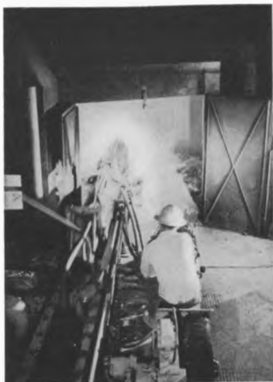
New matte tapping machine is instrumental in reducing costs at the Ray Mines Division smelter.
