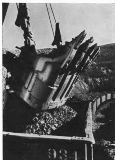
Power shovel loading an ore train at Utah Copper Division's Bingham Canyon mine.
