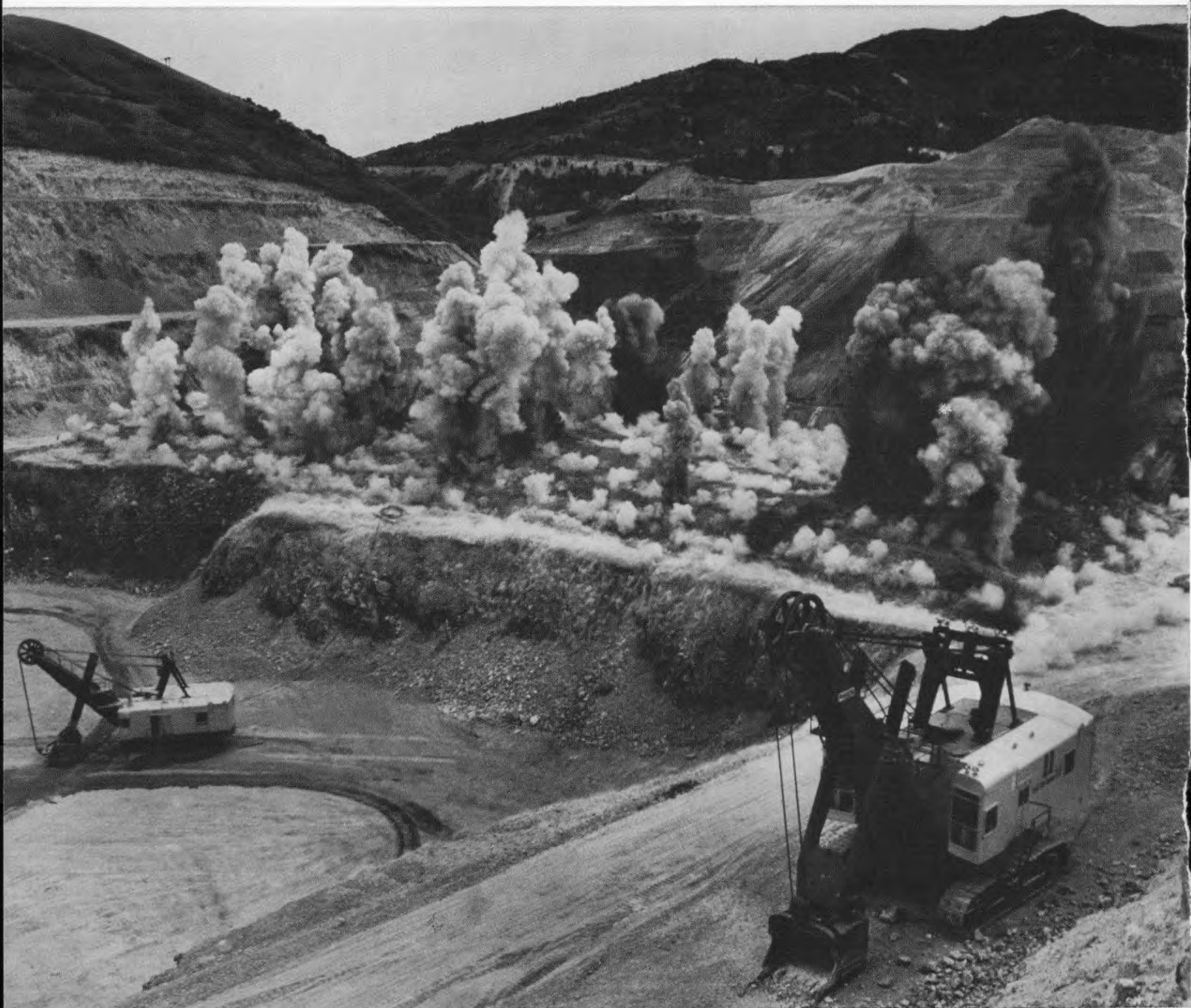
Symbolic of the dynamic expansion program at Utah Copper Division is this 110-hole blast that opens new areas to mining. In the foreground is one of two new 12-cubic yard shovels.
