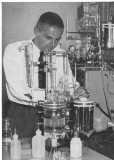
Cell and accessory apparatus used in an investigation of the electrochemical behavior of rhenium metal electrodes at the Ledge-mont Laboratory.
