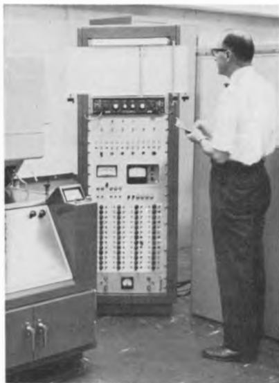
Spectrometer in the Metallurgical Department at Chase Metal Works, Waterbury, Connecticut, determines the composition of copper alloys and records the results.
