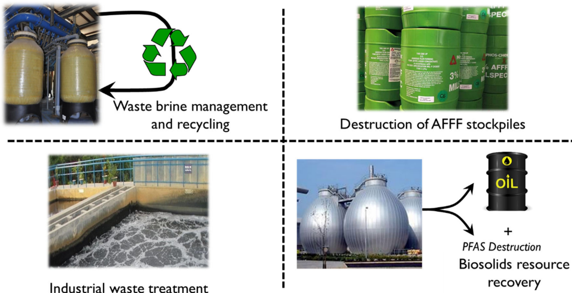
Figure 5.2.1 Illustration of potential applications of the alkaline hydrothermal treatment technology for management of PFASs.
