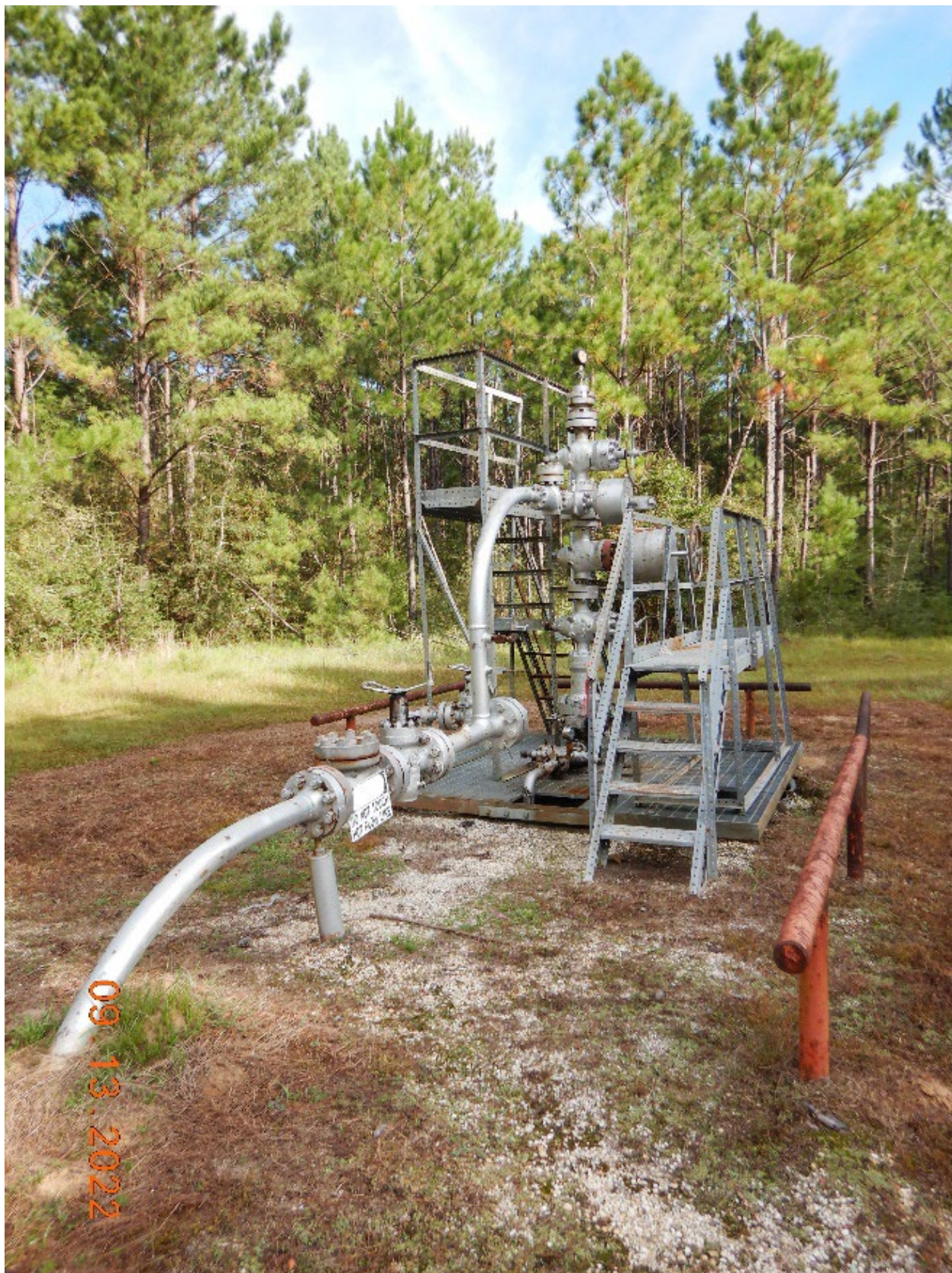
Photograph 5: Looking north, site overview including well head, pressure gauges, valves, and access stairs.
