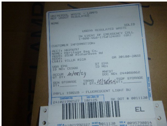
Photograph 23: Label affixed to waste lamp which also indicated accumulation date.
