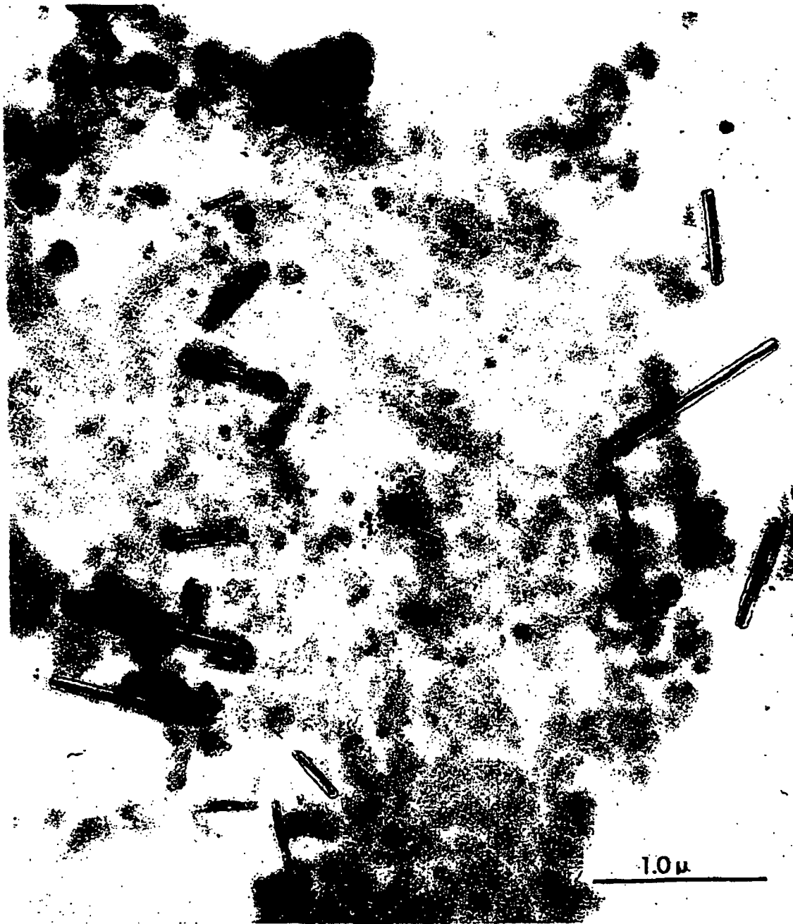
Fig 5.—Chrysotile field in partially digested tissue. Although tissue was electron transmissive, count obtained on screen was 20 compared with count of 31 on photograph. All short and thin fibrils were "missed" on viewing screen.
