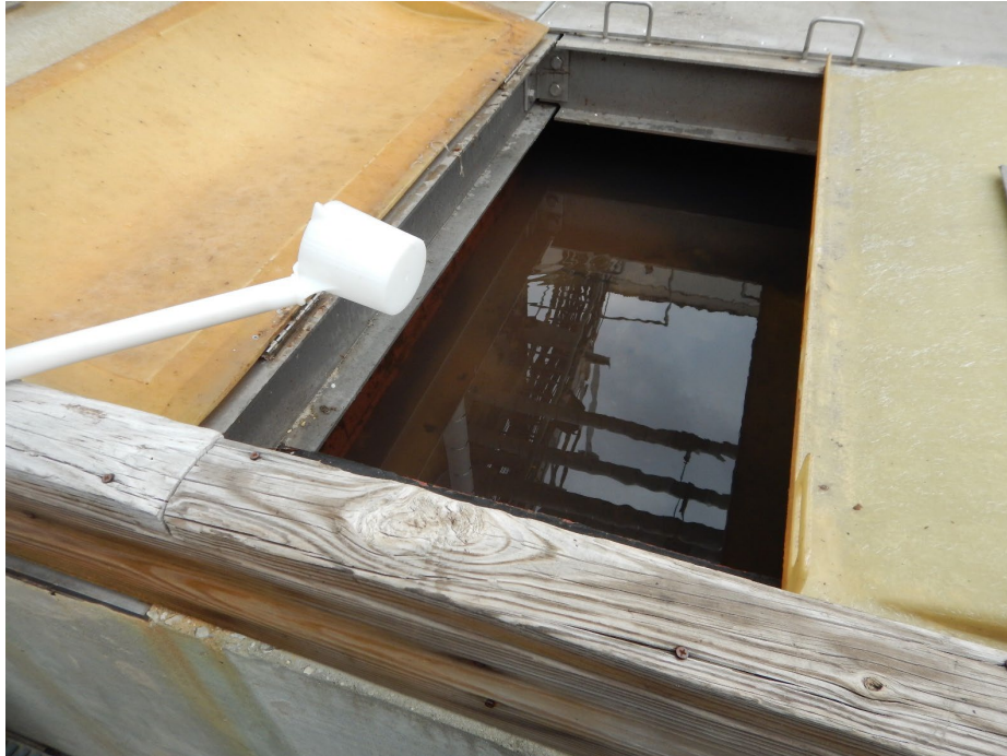
Photograph 60. Sample being taken with a bailer from Tank T56 by Chemours (due to safety reasons).
