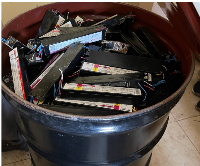
Picture 9 - CHARLES HARDWOOD MEMORIAL COMPLEX, ST. CROIX- At the 2nd Level Main Building Area, there were three (3) 55-gallon black steel drums with lids containing “Ballast” which were not clearly labeled with the words, “Universal Waste-Mercury Containing Equipment,” or dated as required.
