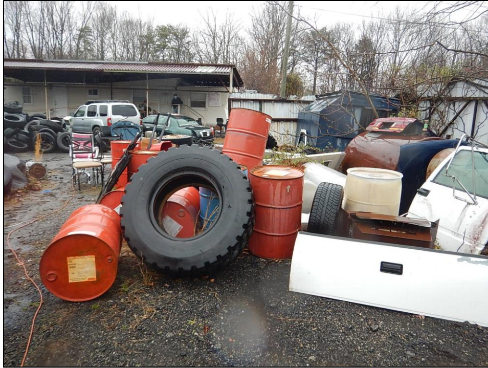
DSCN4130. View, facing north, of uncovered 55-gallon drums, containers, an approximately 275-gallon tank, tires, and various vehicle parts at the southeastern perimeter of the Facility. Note a lack of secondary containment. Facility representatives stated that the drums, containers, and tanks were empty.
