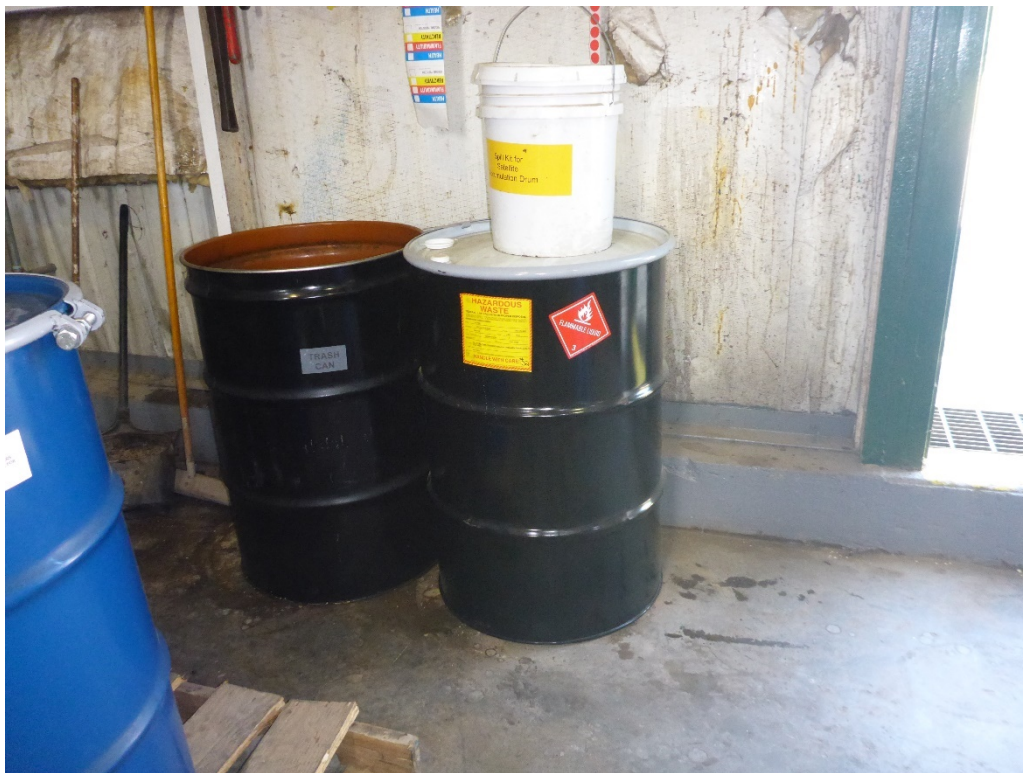
Photo 1: One 55-gallon drum and a 5-gallon spill kit bucket located in the Distillation Area SAA. The drum was closed, labeled D001 / D035 hazardous waste flammable liquids (MEK), and identified with a flammable liquid DOT hazard placard.
