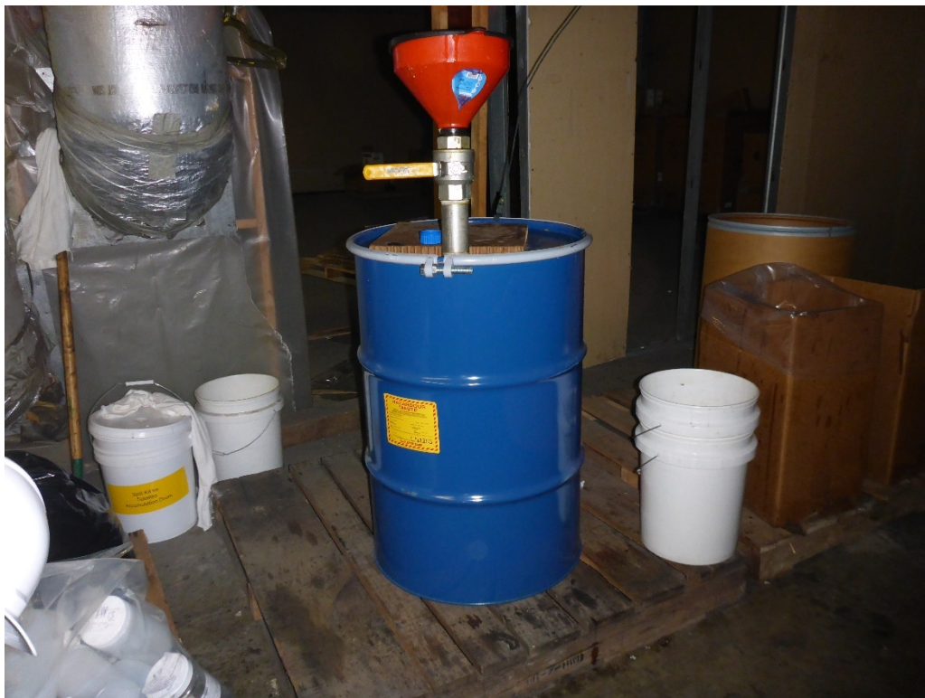
Photo 5: One 55-gallon drum located in one of the QC Laboratory SAAs. The drum was equipped with a closed funnel; it was labeled D001 / F003 hazardous waste flammable liquids; and it was marked as UN 1993 (flammable liquid).
