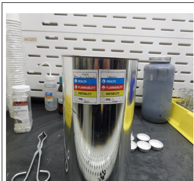
Quality Laboratory. The inspector observed a one-gallon container for waste magnesium perchlorate in a fume hood. The container was not marked or labeled with words Hazardous Waste. Photograph 13 taken at 1:15 p.m.
