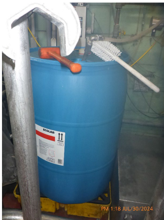
Photograph 1: Sanitary chemical partially on secondary containment pallet at United Dairy.
