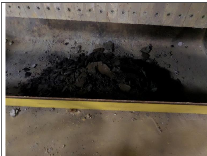
Nickel/Chromium Wastewater Treatment Line. Inspectors observed nickel/chromium solids generated from the filter press were accumulated in a container. Signal representatives indicated the solids are nonhazardous waste. Photograph 5 taken at 10:51 a.m.
