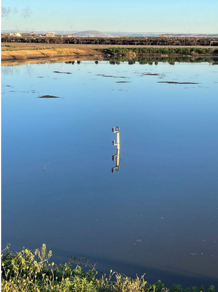
Photo 3. The depth marker in Lagoon 2A with a mark identifying the freeboard level at 5 feet. The pumping level mark is below the surface of the wastewater.
