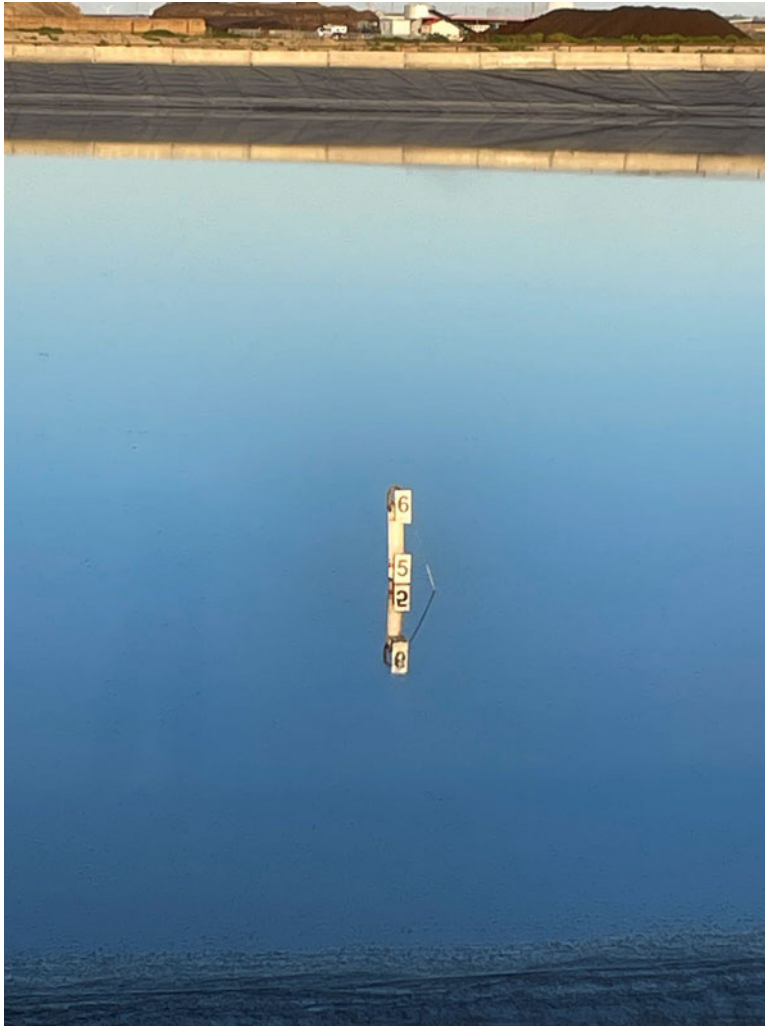
Photo 4. The depth marker in Lagoon 2 with a mark identifying the freeboard level at 5.25 feet. The pumping level mark is below the surface of the wastewater.
