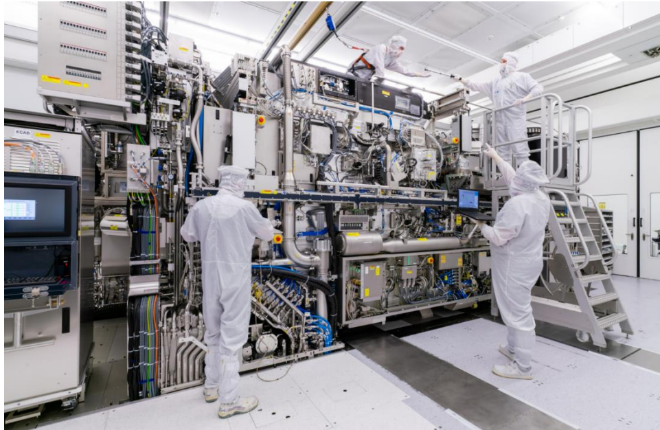
Figure 3: Dutch firm ASML’s latest EUV photolithography exposure tool (Source: ASML).
