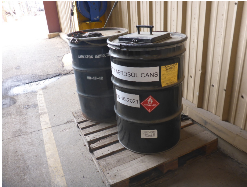
Photo 3: Maintenance Shop SAA for accumulating empty aerosol cans as D001 hazardous waste (acetone, toluene).
