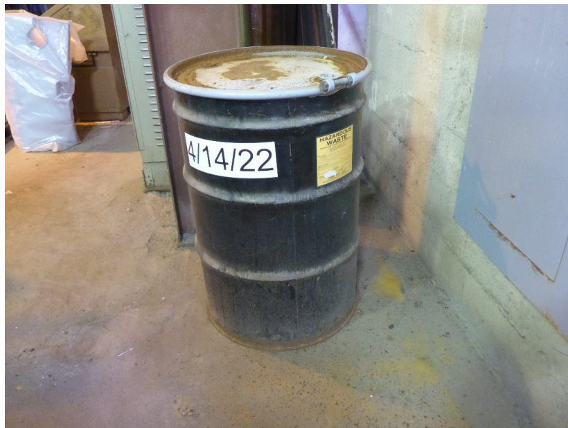
Photo 4: Maintenance Area SAA for accumulating spent grit blast media as D004, D006 hazardous waste solids.
