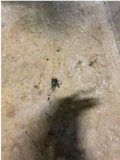
Photo 19: Photo of spilled filter cake on the floor in the area shown in photo 18.
