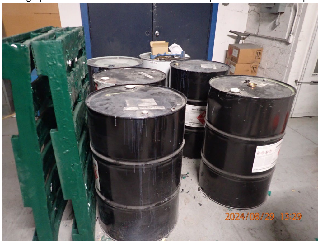
Photograph 15: 55-gallon drums stored at Lepko without secondary containment.
