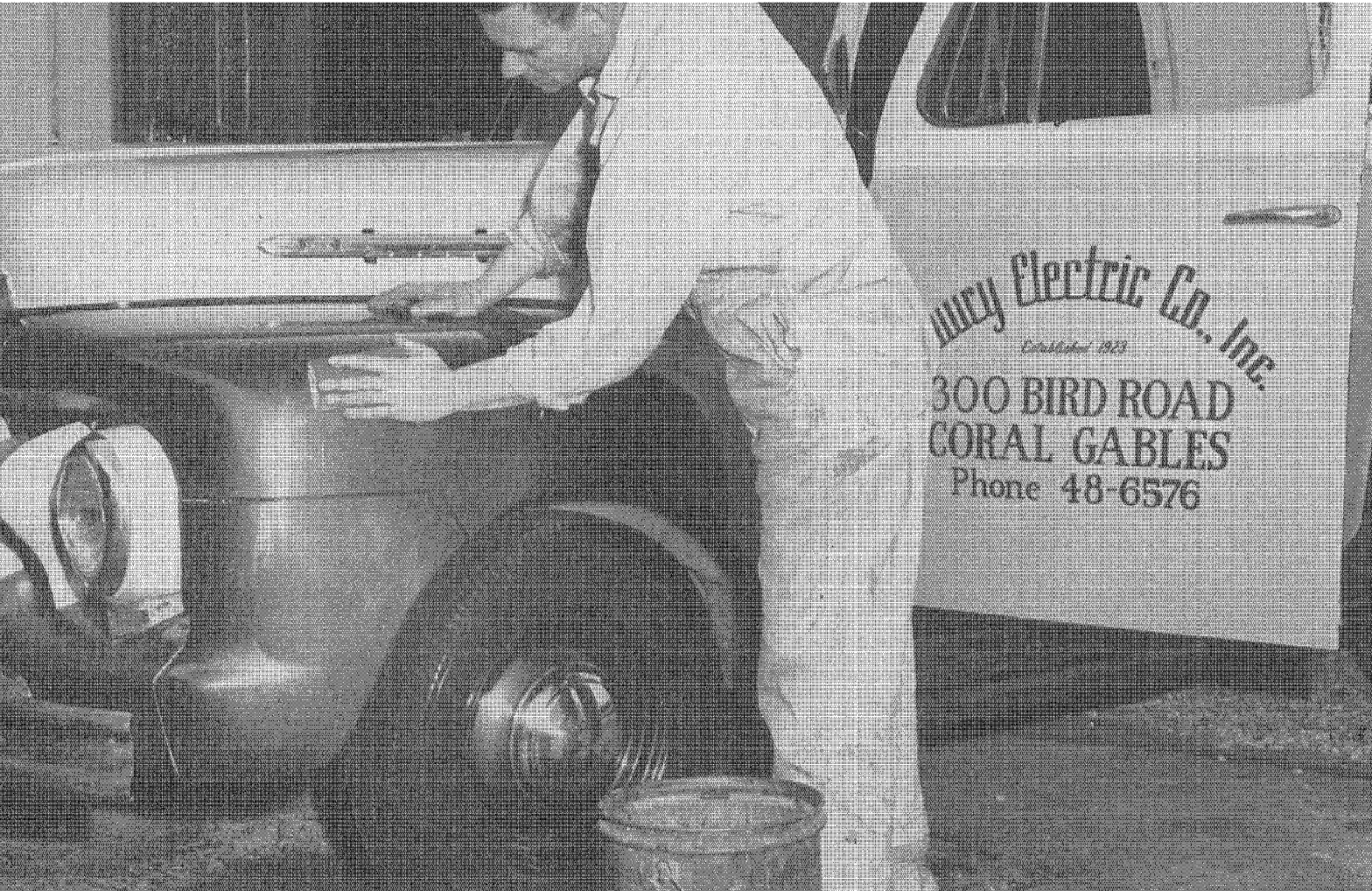
A Lowry Co. truck fender is sanded in preparation for refinishing. The firm specifies "Dulux" for its fleet.
