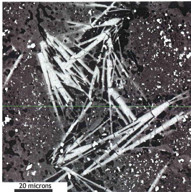
Fig. 13. Backscattered electron image of stilpnomelane needles in a carbonate matrix.
