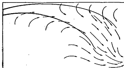
FIG. 6. POSSIBLE SHORT-CIRCUITING WITH RETURN OPENING OPPOSITE SUPPLY
