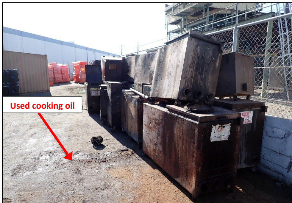
Photograph 2. View, facing south, of used grease traps stored without cover or secondary containment. The containers contained residual amounts of used cooking oil and grease. Note the spilled oil on the ground surface.
