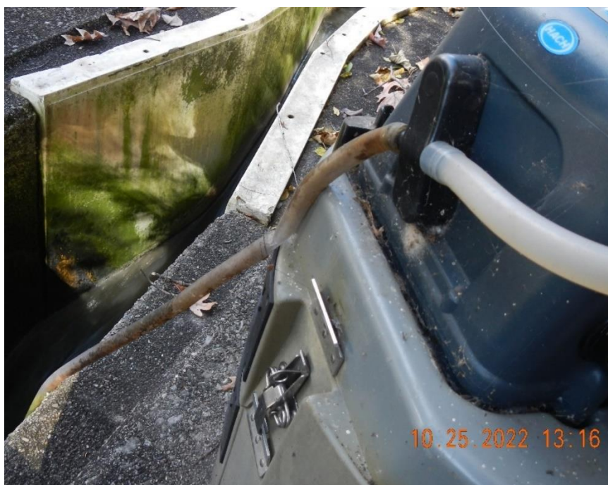
Figure 2. Influent composite sampler. Suction tube was brittle, pinched, and had excessive bacteria lining in the interior of the tube.
