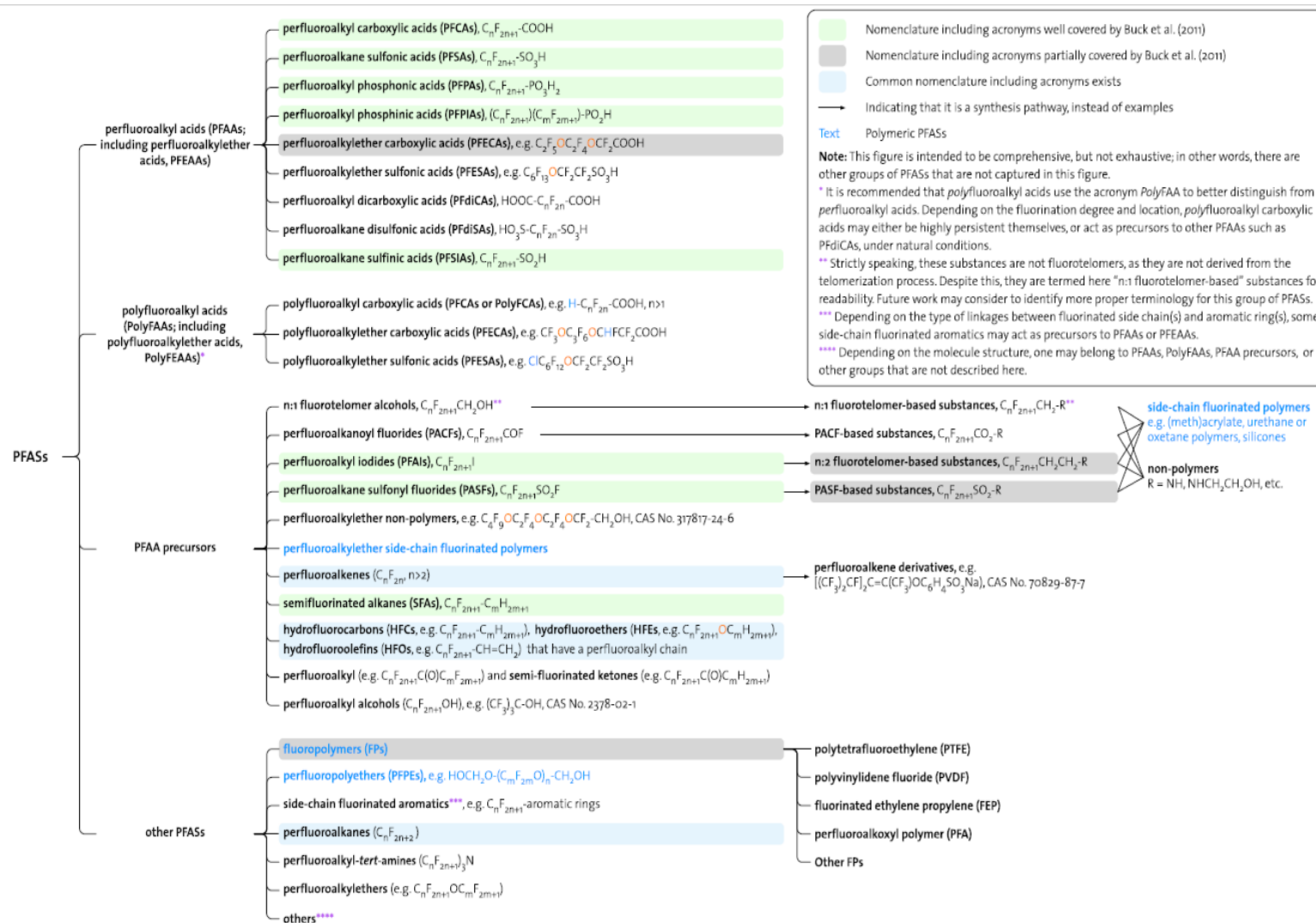
Figure 1: A comprehensive overview of PFAS groups, their structural traits, examples and notes on whether corresponding common nomenclatures (including acronyms) exist. Source: OECD (2021), Reconciling Terminology of the Universe of Per- and Polyfluoroalkyl Substances: Recommendations and Practical Guidance , OECD Series on Risk Management, No. 61, OECD Publishing, Paris.
