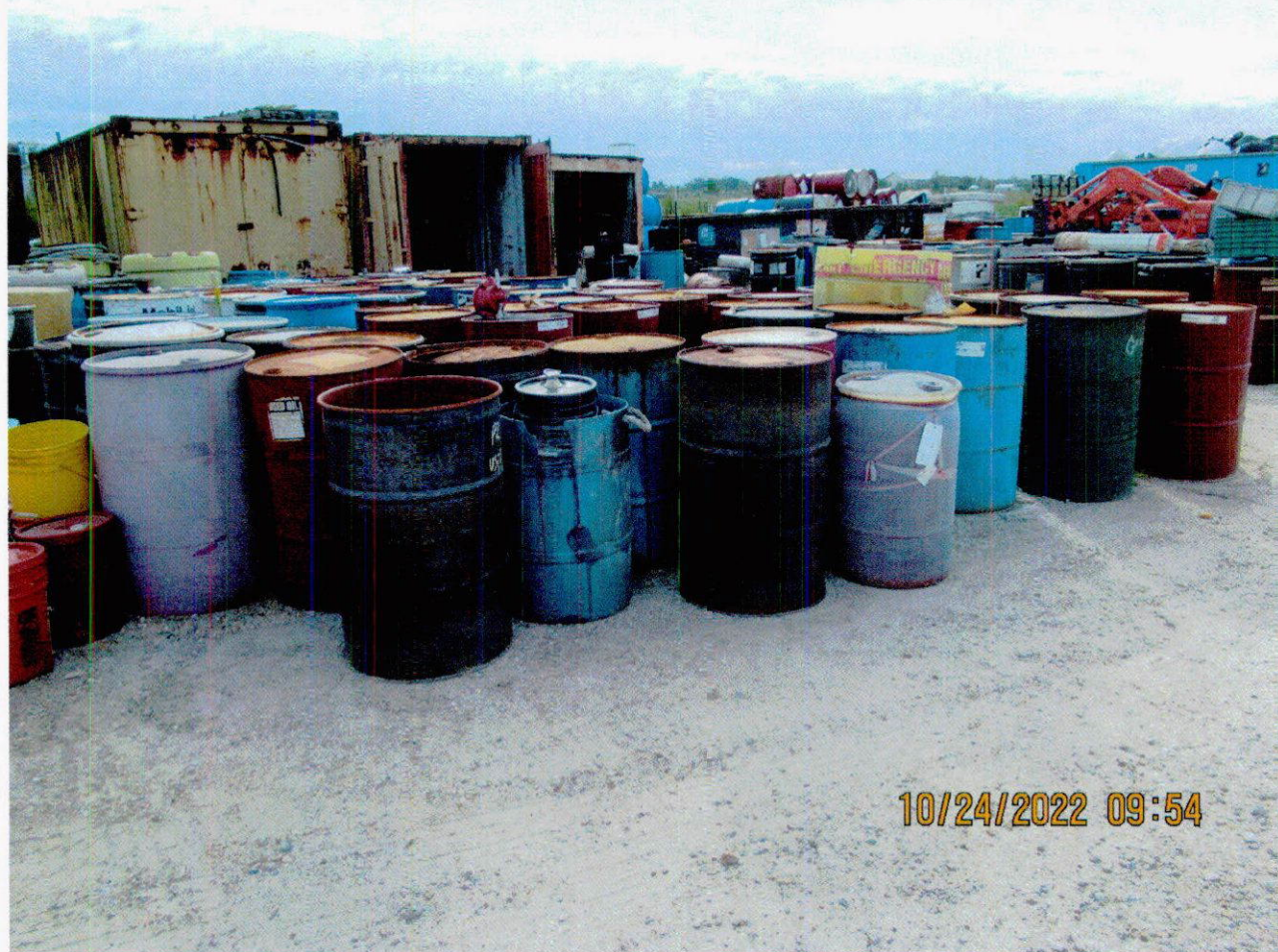
Photo #: 19 Of 81 Date: 10/24/2022 Time: 9:54 AM Description: Several drums of used oil, oily water, and some hazardous waste drums were observed on the east side of the facility. The drums, specifically used oil drums, were on earthen ground and did not have an adequate secondary containment system.
