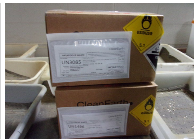
Figure 5: July 11, 2023, 9:34 AM WMF: Room 214-I Inorganic Two (2) 1-foot by 1-foot containers with hazardous waste label, accumulation start date, and indication of the hazards of the contents.
