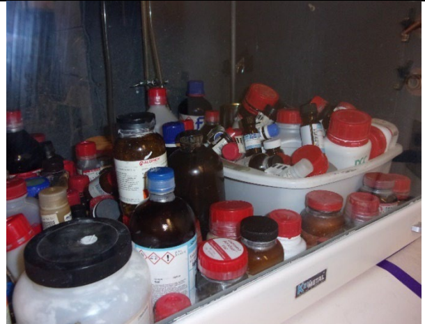
Figure 18: July 12, 2023, 8:59 AM Dabney Hall: Room 842 Fume hood with multiple containers unorganized and placed in a secondary containment bin.
