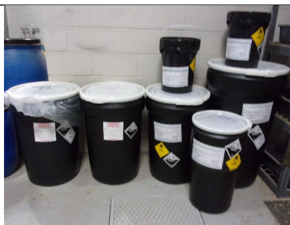
Figure 6: July 11, 2023, 9:41 AM WMF: Room 214-I Inorganic One 55-gallon, three 30-gallon, one 15-gallon, and two (2) 5-gallon lab packs with hazardous waste label, accumulation start date, and indication of the hazards of the contents.
