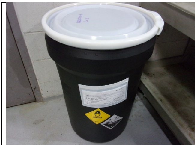
Figure 9: July 11, 2023, 9:47 AM WMF: Room 214-I Inorganic One 30-gallon container with hazardous waste label, accumulation start date, and indication of the hazards of the contents.
