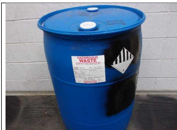
Figure 13: July 11, 2023, 10:06 AM WMF: Room 215 One 35-gallon container with hazardous waste label, accumulation start date, and no proper indication of the hazards of the contents.
