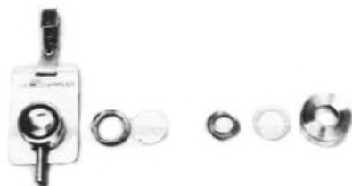
Figure 4.6 Sampling head for inhalable dust (after Hinds)
