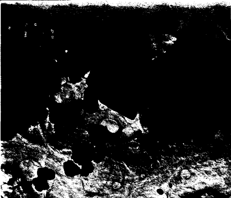
FIGURE 1—Electron micrographs (x24,000) of commercial 50 lb. offset containing 1.68 per cent \text{TiO}_2 and 22.5 per cent clay. Sheet at left does not contain asbestos and has densely packed agglomerates of \text{TiO}_2 (black) and clay (gray, angular) with large surrounding voids. Sheet at right contains 1.5 per cent asbestos and has a more uniform distribution of \text{TiO}_2 and clay. Thus, latter structure provides better light-scattering efficiency.
